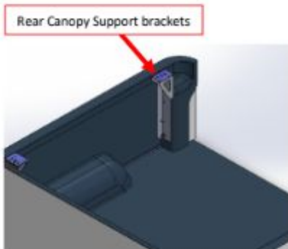
Figure 7: Rear Canopy Support Bracket Position
