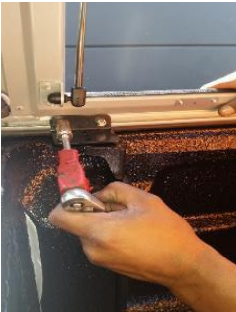
Figure 21: Tightening Universal bracket to Canopy
