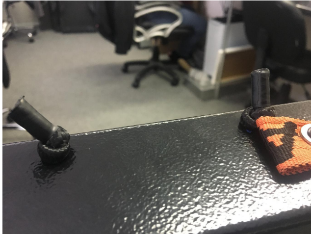
Figure 12: Insulation Taped Ends
