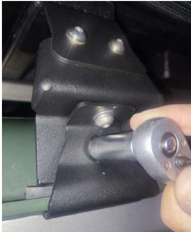
Figure 7: Completing gutter mount fitment
