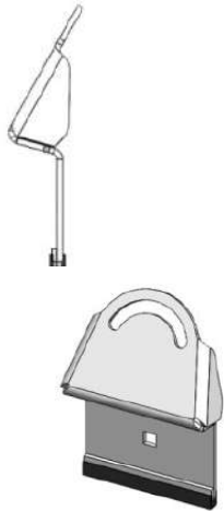
Figure 2: Gutter Mount with 5mm rubber channel
