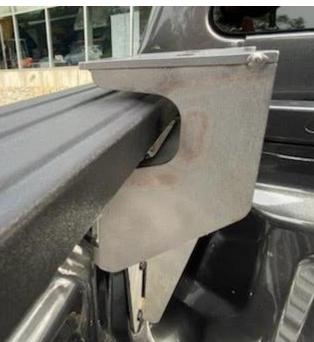
The nut and washer, that need to be located from the underside, are indicated above. The working space between the load bed walls, and the Khaya frame is very tight. It is advisable to use a 13mm ring spanner, and using a small piece of adhesive tape, locate the nut and washer in the ring spanner. This will ensure that it does not fall out, into the load bin, during installation.
